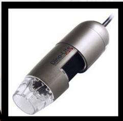
*Microscopic cameras are used to examine contaminants in oil such as, metal debris, general contamination, heavy contamination, water ingress and other contaminants.*
